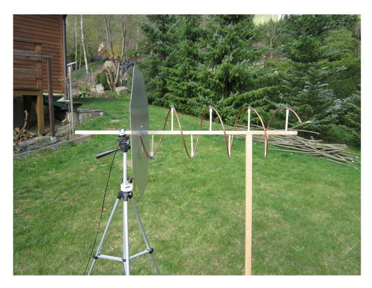
An antenna for tracking <u>TT7 High Altitude Baloon</u> on 434MHz. Linked article includes Smith Charts and other modeling used to design the antenna. It then goes into creating this antenna.
